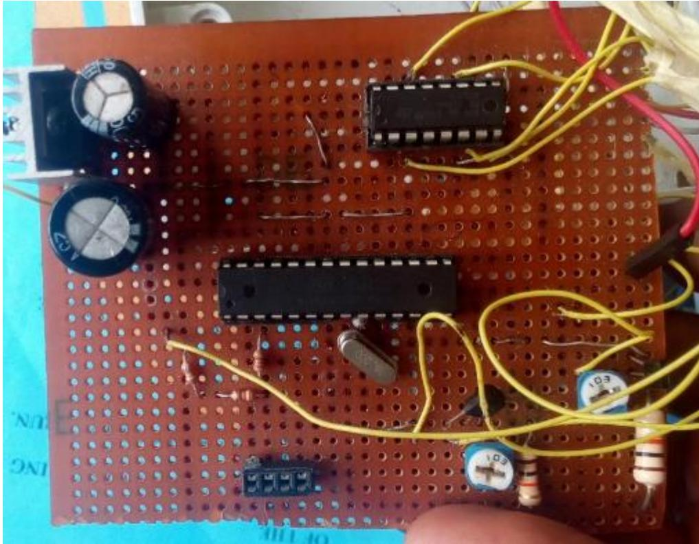
**Figure 7 Implementation of the communication unit**
