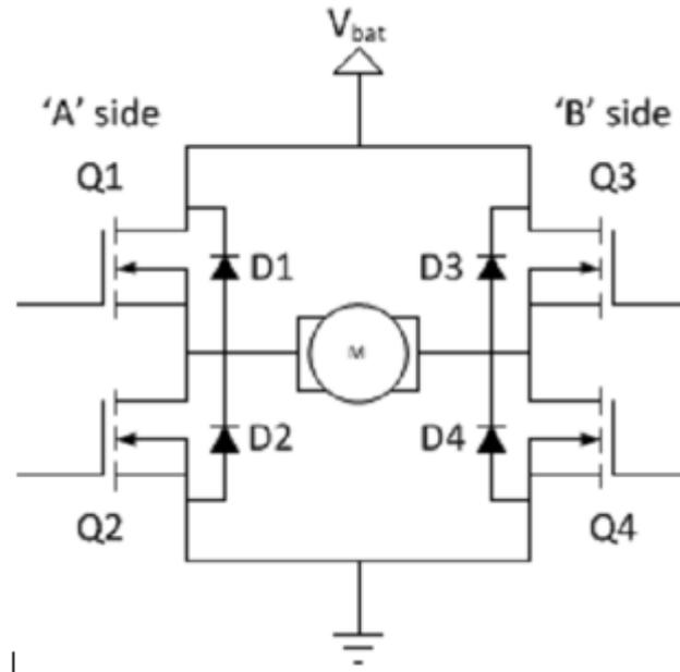
**Figure 3 H-Bridge circuit diagram**
