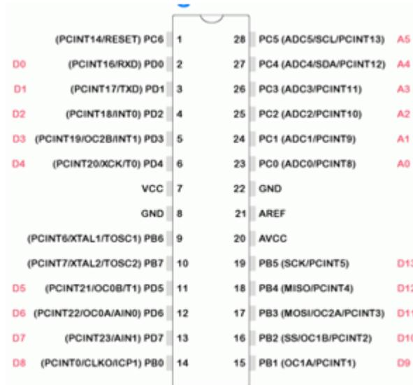
**Figure 2. Atmega328P micro-controller**
