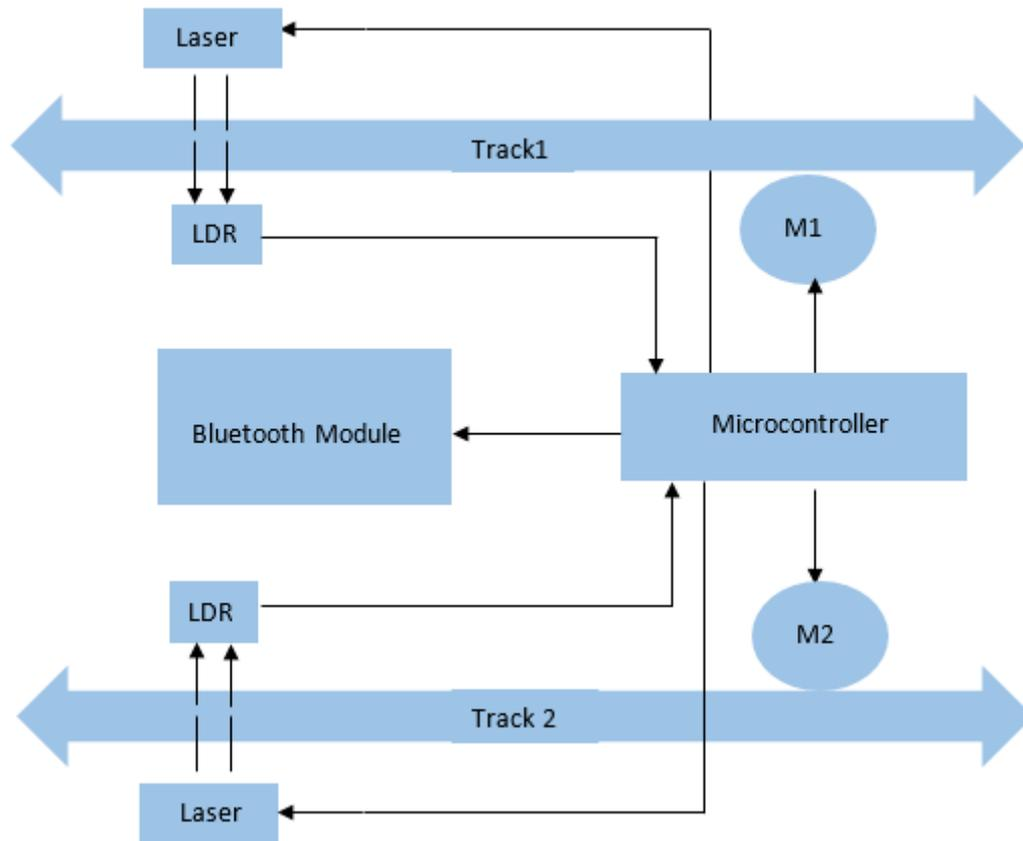
**Figure 1: Block diagram of the system design**
