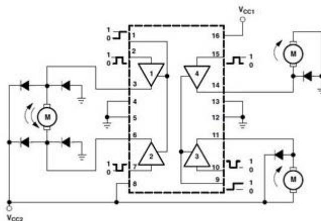
**Figure 4 Functional Block Diagram of the L293D**
