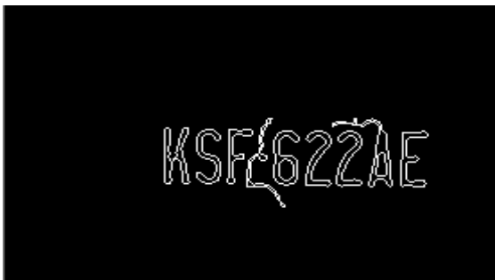
Figure 6: Filtered contours with defined dimensions (Area, weight, and height)
