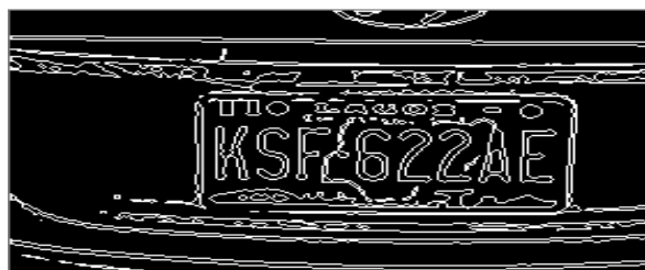
Figure 6: Filtered contours with defined dimensions (Area, weight, and height)
