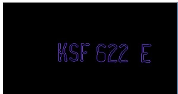
Figure 6: Filtered contours with defined dimensions (Area, weight, and height)
